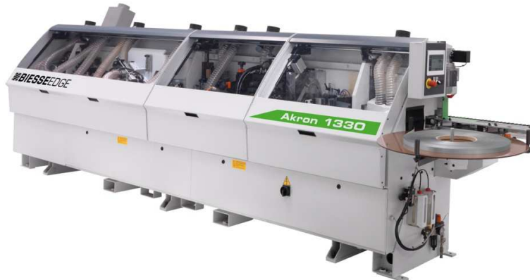
Autoamtic edgebanding machine Akron 1300
